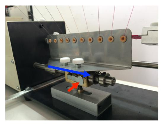
The traverse guide plate is tightened by the white head screw.
