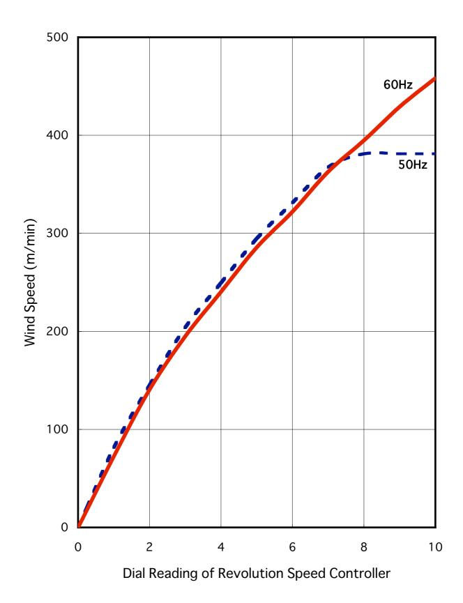
Marusan Portable Winder Winding Speed for CM-2HT
